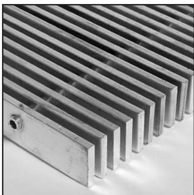
P-6-4, 1" x 3/16", Smooth Surface, 3/8" bearing bar centers; 4" cross bar centers
