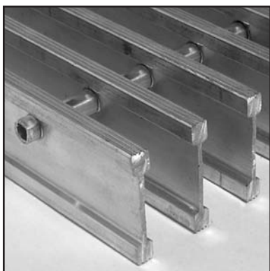
P-15-4, 1-1/2" I-Bar, Grooved Surface, 15/16" bearing bar centers; 4" cross bar centers
